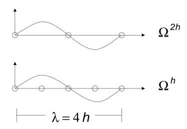
• In particular, GS (and other relaxation schemes) very effective for reducing error/residual components on  $\Omega^h$  that cannot be represented on a 2:1 coarser mesh,  $\Omega^{2h}$ , i.e. that are above the Nyquist limit on  $\Omega^{2h}$ , i.e. with wavelengths,  $\lambda < 4h$ ; generally takes some constant (i.e. h-independent) number of sweeps to reduce magnitude of high-frequency components by given factor
